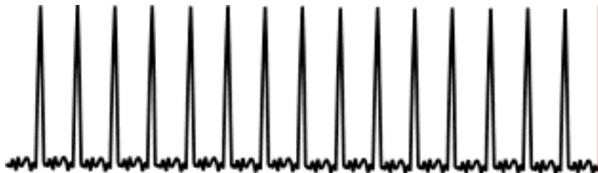
Figure 4 Wideband spectrum of HF digital voice hopper, accumulated over time.
