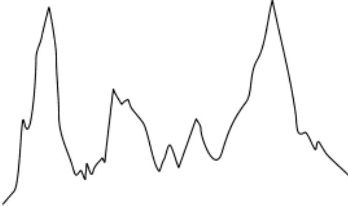
Figure 1 - Typical HF Spectrum Occupancy
